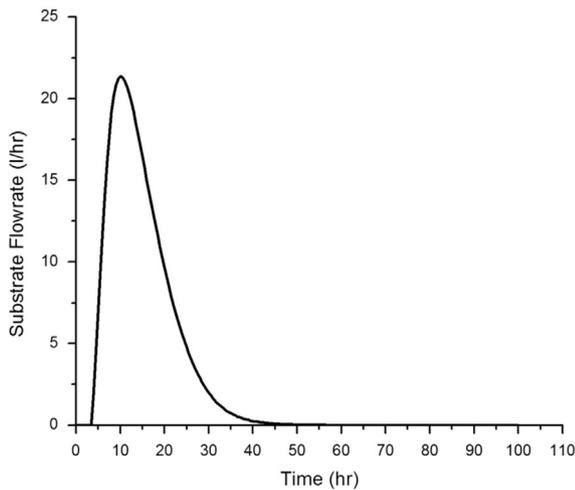
Fig. 4. Optimal control variable profile in the fermentation case-study.
