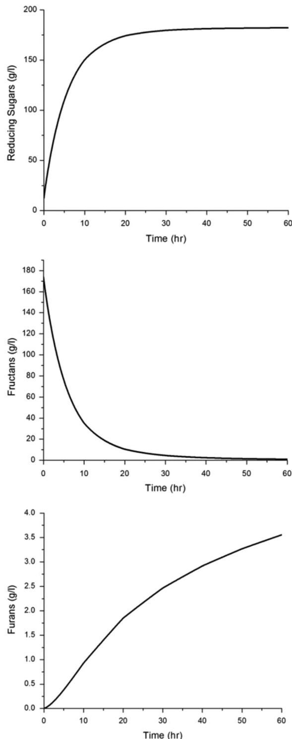
**Fig. 6.** Optimal profiles for the state variables in the thermal hydrolysis of Agave.
