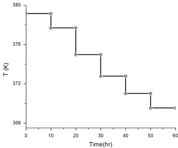
Fig. 7. Optimal temperature (control) profiles for the thermal hydrolysis of Agave.
